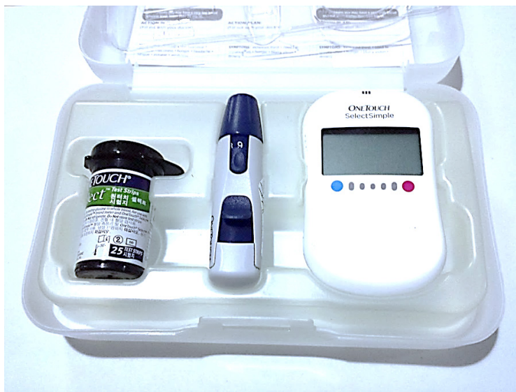
Figure 5. Photo of the One Touch® Select Simple™ Blood Glucose Monitoring System (OneTouch® Select® Test Strips, Lancing Device, OneTouch® SelectSimple™ Meter) that was used in measuring the blood glucose levels of the rats.
