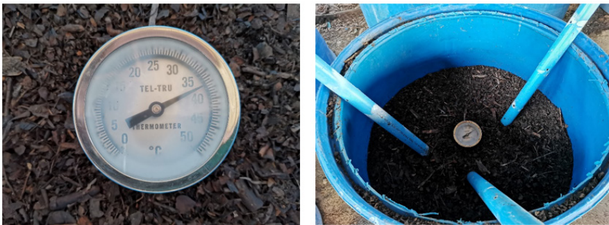
Figure 3. A thermometer with a 30 cm stem was used to measure the temperature of the substrate weekly.
