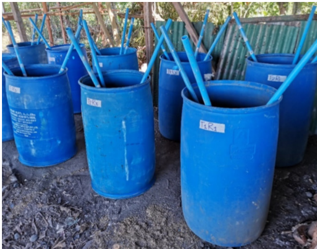
Figure 2. Perforated barrels were used to contain the substrate, with perforated PVC pipes utilized as aerators for the decomposing feedstock.
