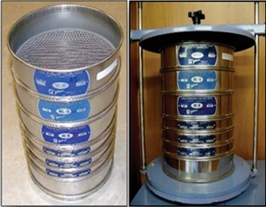
Figure 5. The sieve series used in grain-size analysis to determine the soil composition
