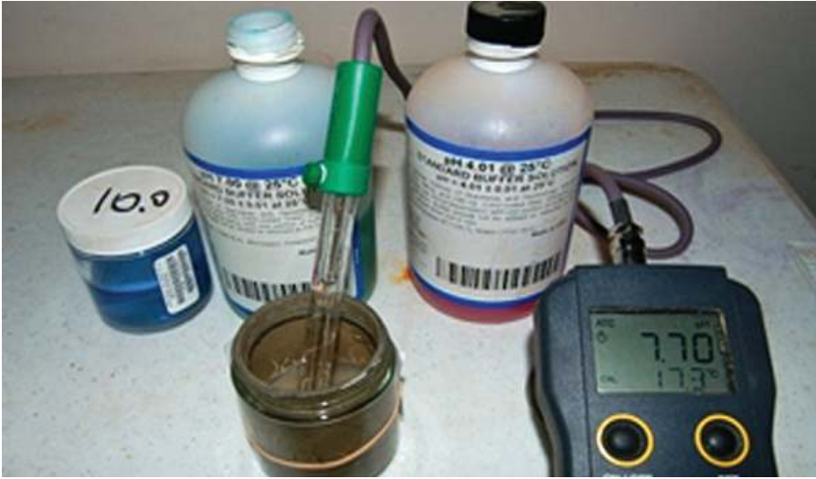
Figure 7. The portable pH meter used to measure soil pH.
