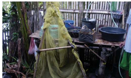
Figure 8. Specialized electro-fishing gear. Electrodes are attached to the fine net. The contraption operates like an electrified scoop-dredger.
