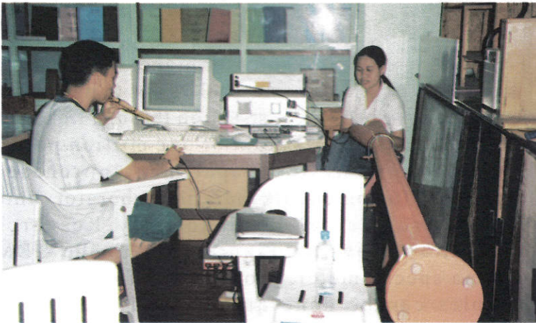
Figure 8 BS physics students analyzing the sound of a pipe with a sound sensor and the SR 760 Frequency analyzer.
